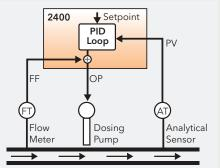
2400 series Feedforward control is excellent for chemical dosing applications
