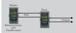
Using Eurotherm setpoint retransmission over PDS communications it is possible to use two 2400 controllers as a cascade control system with the output of the first (or master controller) forming the setpoint of the second (or slave controller).
