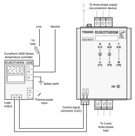
Polarity insensitive DC logic signal
