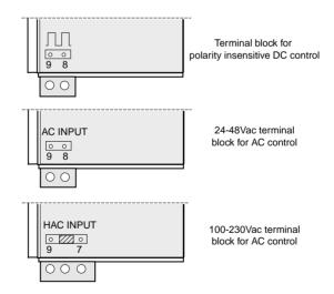
Figure 3-2 Control terminal block labels
