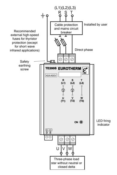
Figure 3-1 Power and safety earth wiring for a load connected in 'star without neutral' or in 'closed delta' (3-wire configuration)
