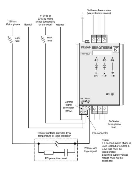
Figure 3-6 Example of wiring for 230 Vac AC signal and fan (63A)
