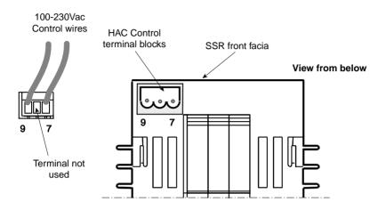
Figure 3-4 Control terminal block for HAC code
