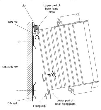
Figure 2-3 DIN rail mounting for TE200S solid state relay
